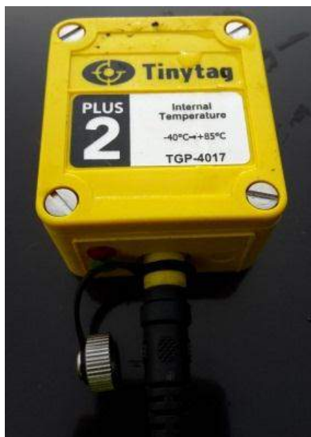
Figure 21: Temperature sensor and data logger, Tinytag
