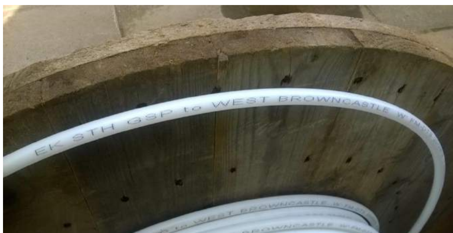
Figure 7: Embossed micro-duct – West Browncastle (white)
