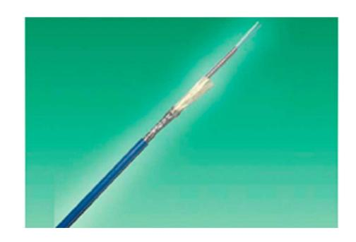
The AT cable is designed to be lightweight and flexible making it easy to handle and install and with a very fast thermal response time. Inaddition, the dual stainless steel and Kevlar protective layers provide excellent mechanical, tensile and pressure resistance (IP68 waterproof rating).
