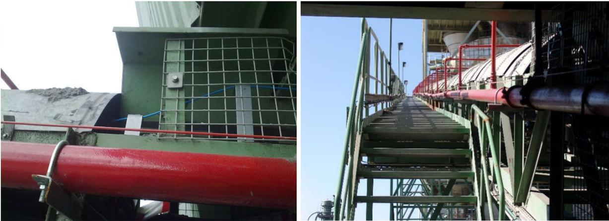
*Path of the sensor cable in relation to the conveyor belts*
