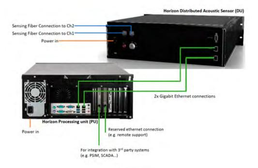
The DU connects to the fiber optic sensing elements and contains all the optoelectronics to interrogate the fiber optic and data acquisition components to acquire the data. The PU is based on a high-performance industrial PC and carries out the classification algorithms (including the DNN machine learning) as well as the user interface.
