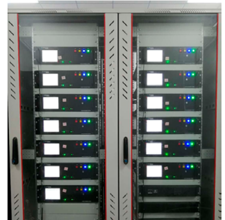
Figure 4: The 13 FireLaser DTS systems in the cabinet
