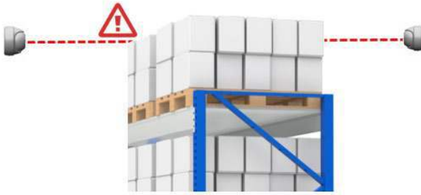
Beam detectors blocked by objects
