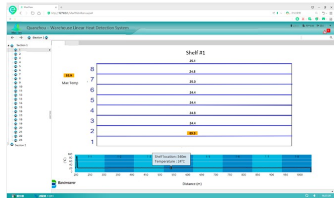
Figure 12 – Screenshot profile view of rack 1 within warehouse
