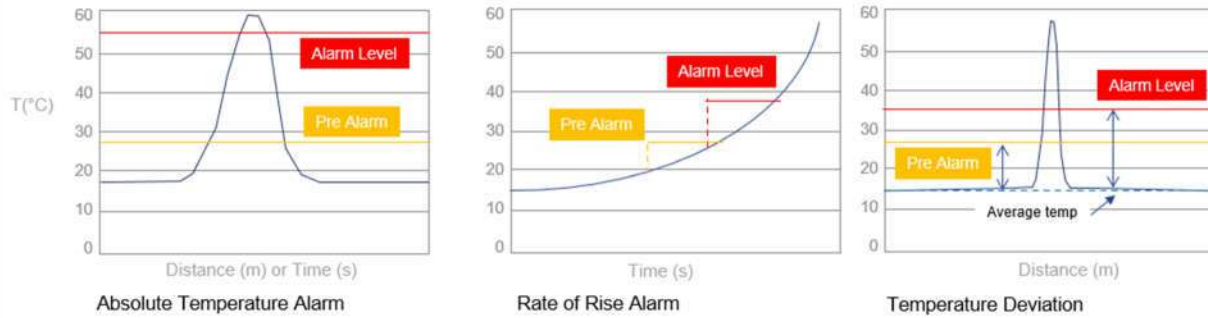
Figure 2 - Smart alarming with fiber optic linear heat detection systems
