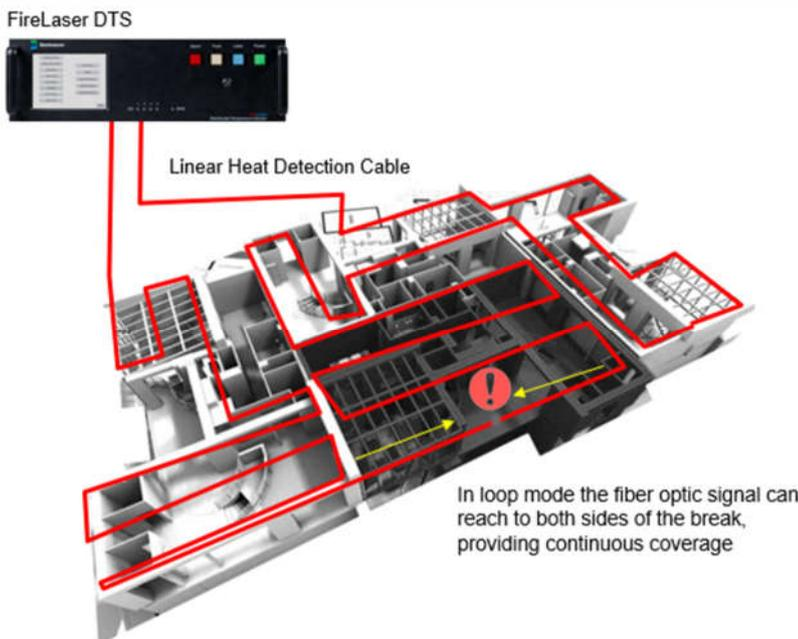
Figure 7 - Loop redundancy example
