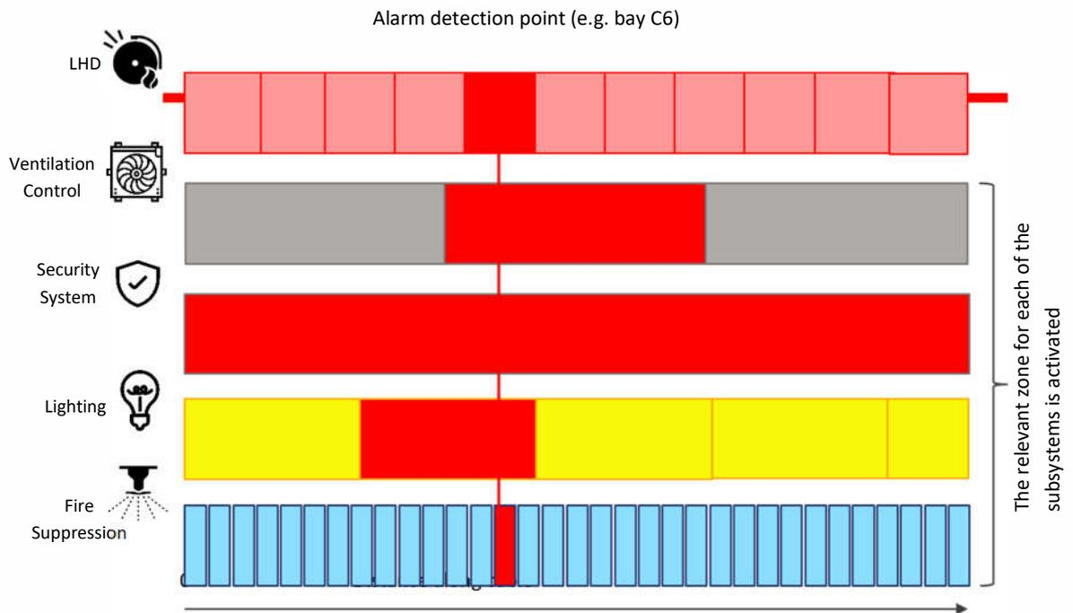
Figure 3 - Example of smart zone configuration
