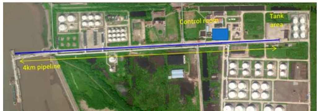
Figure 1: Details of pipeline and sensing cable within propylene plant
