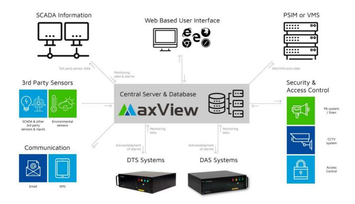
MaxView is an extremely versatile platform and can interface with multiple 3rd party platforms including SCADA, DCS, CCTV, PSIM, VMS, etc. as well as a number of proprietary 3rd party systems.
