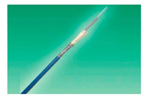
The AT cable is designed to be lightweight and flexible making it easy to handle and install and with a very fast thermal response time. Inaddition, the dual stainless steel and Kevlar/aramid yarn protective layers provide excellent mechanical, tensile and pressure resistance (IP68 wa terproof rating). It is a very similar construction to the standard FireFiber AT but with an additional layer of Kevlar.
