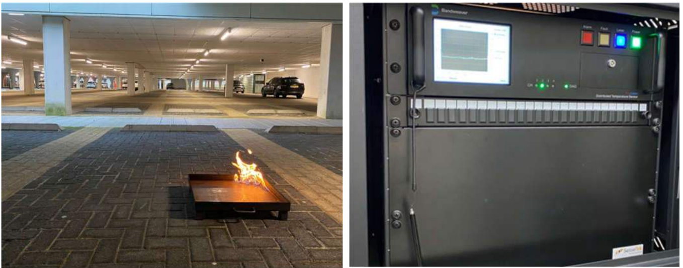
Figure 3 - Photo of fire pan test and the FireLaser LHD system
