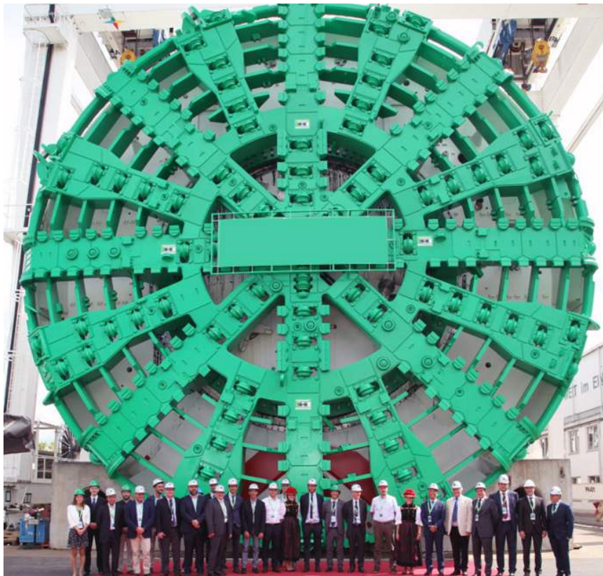
Figure 1 - The tunnel excavation cutter
