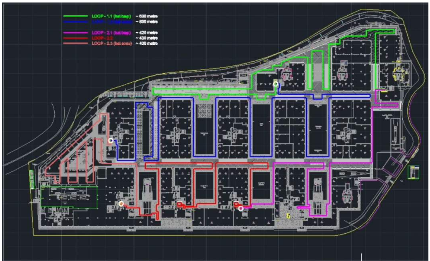
Figure 4 - Fiber route within mall
